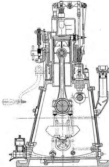
Figure 3. Variable Compression Ratio CFR Engine.<sup>19</sup>
