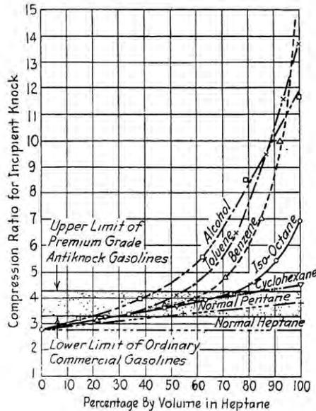
Figure 6. Detonation Characteristics of some Antiknock Standards.
