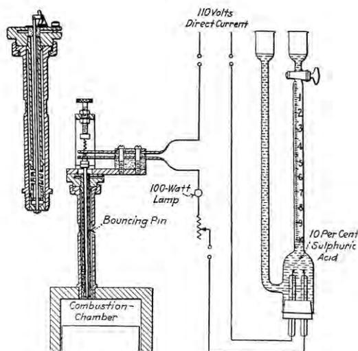
Figure 4. Original Bouncing Pin Knock Detection Equipment.<sup>20</sup>
